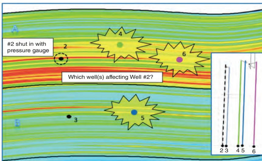
This diagram shows the location of well #2 in relationship to wells #4, #5, and #6. Because those wells were completed around the same time, the operator was left guessing which one caused a frac hit. *Source: EP Energy.*
