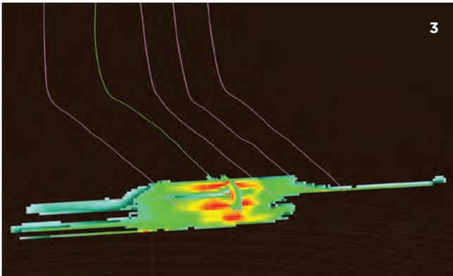
Frame 1 of a modeling sequence shows a hydraulic fracture may contact a depleted reservoir section of multiple parent wells—inducing a frac hit across the pad. A larger fracture network develops around the child well only after the fracturing fluids have filled that depleted area, shown in frames 2 and 3. *Source: Barree & Associates.*
