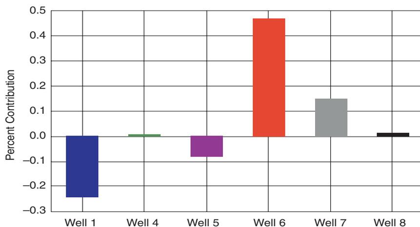
Using diagnostic firm Biota Technology’s DNA surveillance and analysis, EP Energy conclusively determined that well #6 was responsible for frac hits on well #2. Source: EP Energy.
